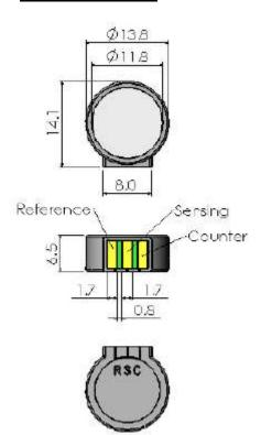
All dimensions are in millimeters. All tolerances are ±0.2mm.
