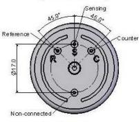
All dimensions are in millimetres mm. All tolerances are +/- 0.2mm.
