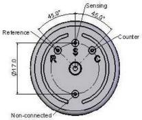
All dimensions are in millimetres mm. All tolerances are +/- 0.2mm. Note: PCB sockets are recommended for the sensor pin connection. Soldering or using glue with the sensor should be avoided and will invalidate warranty.
