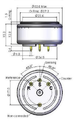
All dimensions are in millimetres mm.
