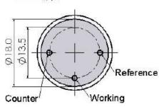
All dimensions are in millimetres mm. All tolerances are +/- 0.2mm.
