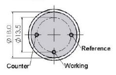
All dimensions are in millimetres mm. All tolerances are +/- 0.2mm.
