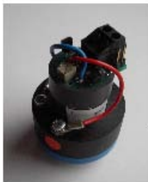
Figure 2. Top view O 2 SL Oxygen sensor with 4-20mA transmitter and installation kit. Part no. 2112B4532
