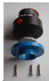
Figure 3. Components O 2 transmitter with sinter metal disc and blue installation ring
