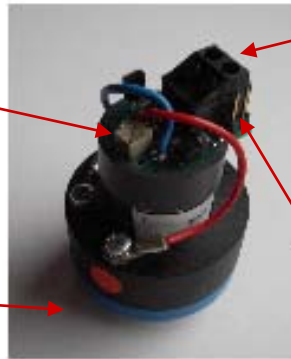
Figure 5. Instructions O 2 SL Oxygen sensor with 4-20mA transmitter and installation kit. Part no. 2112B4532
