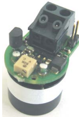
Figure 1. NO 2 sensor with 4-20 mA transmitter
