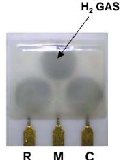
A RAW sensor is part of a wafer which contains 48 RAW sensors. Every wafer is gas tested prior to shipment. The sensors are separated through pre-manufactured break lines as shown on the next page's illustration. The separation process is very easy if the order is followed carefully.
