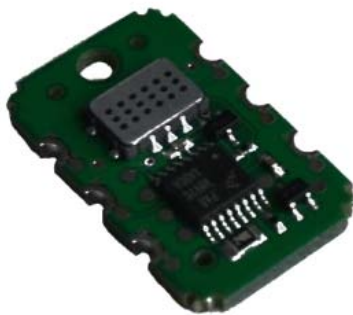
C5 miniature integrated sensor board for VOCs & CO2 equivalent monitoring. Part no. 2112BC500
