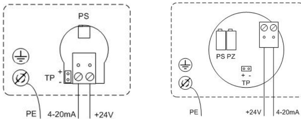
**Connection diagram.** Left: version with two-electrode sensor; right: version with three-electrode sensor; PE, potential earth; PS, potentiometer span for setting the span; PZ, potentiometer zero for setting zero (three-electrode sensor only); TP (+) (-), test pins for connecting the voltmeter; 2 polarized screw terminals for power supply (+24 V DC) and measured signal output (4-20 mA).
