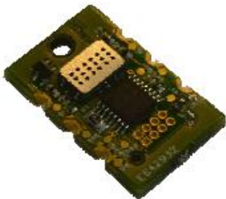
C5 miniature integrated sensor board for VOCs & CO2 equivalent monitoring. Part no. 2112BC500
