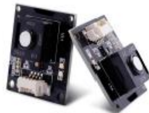
SS Micro TX UART or i2c miniature precalibrated pluggable transmitter, part no. 2112B0127905
