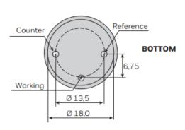
All dimensions are in millimetres mm. All tolerances are +/- 0.2mm.
