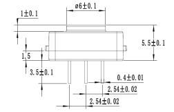
All dimensions are in mm. Tolerances are +/- 0.10mm unless otherwise stated.
