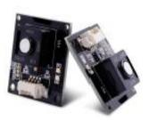
UART or i2c miniature precalibrated pluggable transmitter, part no. 2112B0127502
