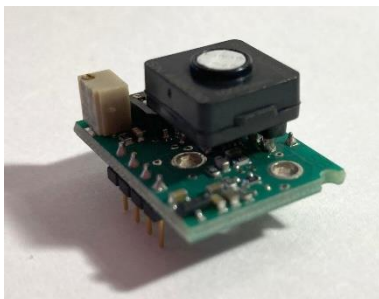
SS PCB Voltage and i2c miniature precalibrated pluggable transmitter, with onboard temperature measurement and life test capability, part no. 2112B019900
