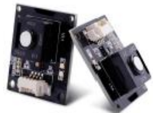
SS Micro TX UART or i2c miniature precalibrated pluggable transmitter, part no. 2112B01278010
