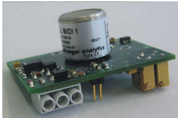
Figure 2. LEL sensor plugged on 4-20 mA transmitter
