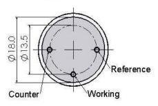
All dimensions are in millimeters. All tolerances are ±0.2mm.
