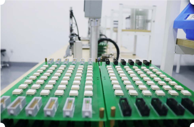
Sensor Production Test
