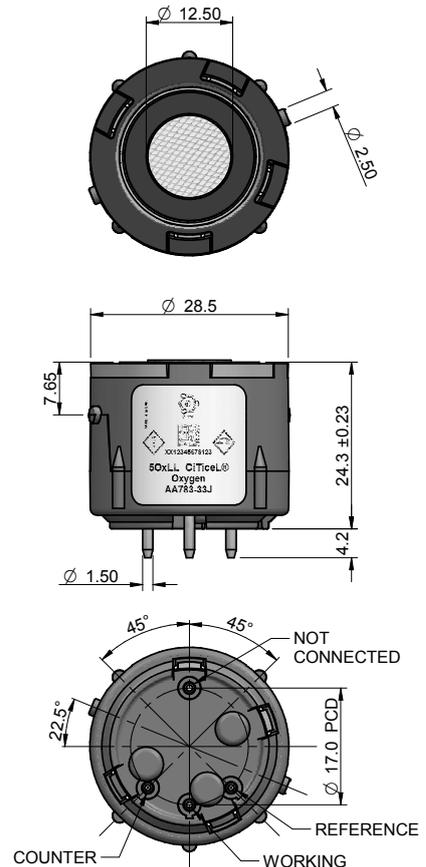
All tolerances ±0.15 mm unless otherwise stated. DO NOT solder to pins.
