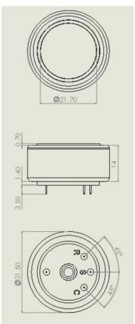
All dimensions in millimeters (± 0.1mm)
