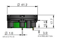
All dimensions in mm All tolerances ±0.15 mm unless otherwise stated 3SF shown with side tags and tin pins
