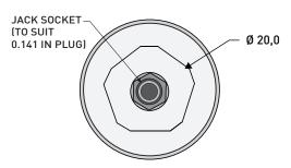
**Important Note:** Connection should be made via recommended mating parts only. Soldering to the sensor will damage it and invalidate the warranty.
