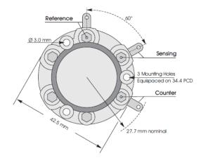
All dimensions in mm All tolerances ±0.15 mm unless otherwise stated 3FD shown with side tags and tin pins
