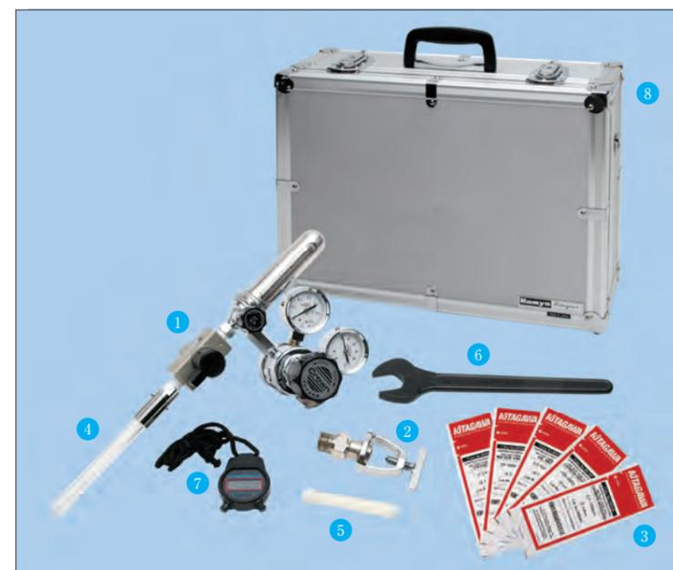
Impurities in breathing air for respiration can adversely affect human health. The kit is designed to measure these contaminants in SCBA, SCUBA and other pressurized breathing air cylinders, as well as directly from the outlet of an air compressor or purifier. The kit easily measures five components within minutes : carbon monoxide, carbon dioxide, oil mist, water vapor and oxygen by aerating the detector tube with an exclusive reducing valve from the breathing air source.
