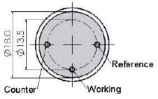
All dimensions are in millimetres mm. All tolerances are +/- 0.2mm. Note: PCB sockets are recommended for the sensor pin connection. Soldering or using glue with the sensor should be avoided and will invalidate warranty.
