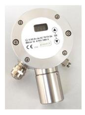
The modular design of the sensor allows it to be equipped with a catalytic sensor (pellistor) for determining the concentration of explosive gases and vapours, or with an electrochemical sensor for toxic gases depending on the variant. The concentration is output from the 4-20mA interface, for further processing.
