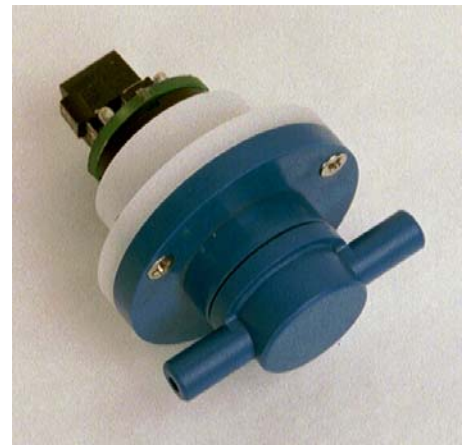
Figure 5. EXAMPLE: ECO-Sure CO sensor and 4-20mA transmitter (part no. 2112B1005) assembled with installation kit (part no. 2112B1002) and plugged into test gas cap (part no. 2112B1010). This unit is ready for installation into housing or a panel (please note: sensor holder is now black).
