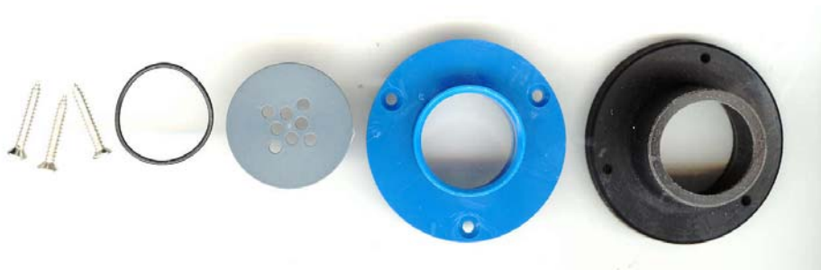
Figure 7. NO2 Installation Kit Components (left to right) for NO2 sensors. Part no. 2112B1012 Screws, small o-ring, plastic sensor protection disc, sensor fixing ring and sensor holder.
